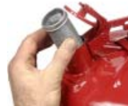
Flame arrestor screen inside spout prevents flashback
