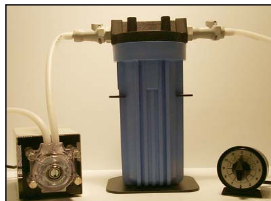
Large volume system includes peristaltic pump, timer, cartridge & stand.
